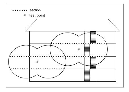
Figure 7: Typical radio coverage areas in a building
