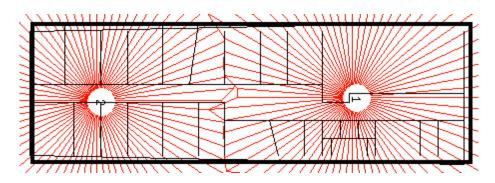
Figure 11: Radio areas of two base station covering the building with stronger walls
