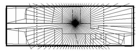
Figure 10: Radio area of one base station if the walls have stronger attenuation
