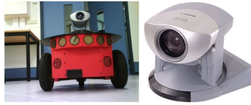
Fig. 5 Experimental set-up: external view of the used mobile platform (left) and a more detailed view of the camera (right)
